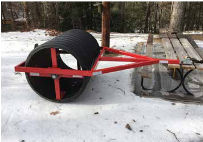
A new roller/packer fabricated by the "Burnache Boys" for the Burgy Bullets will make for smooth trails.
