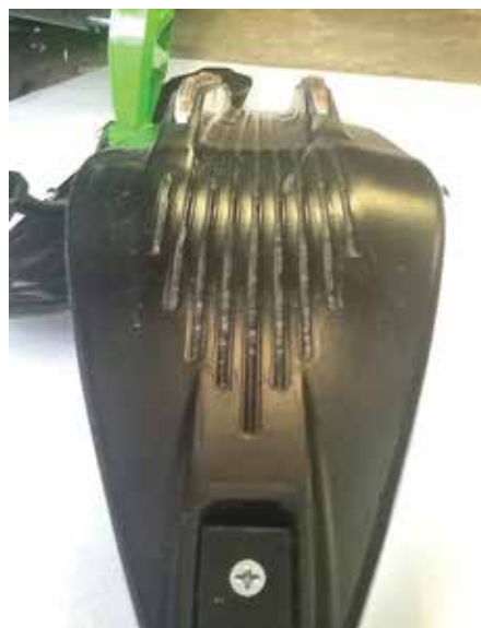
The Gen III carbides are not pushed out to the edge of the ski as they were in previous versions. Note the deep keel.
